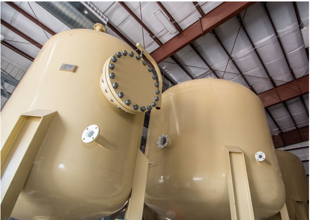
Figure 3: Ion Exchange Columns within the completed CPP, Wyoming USA
