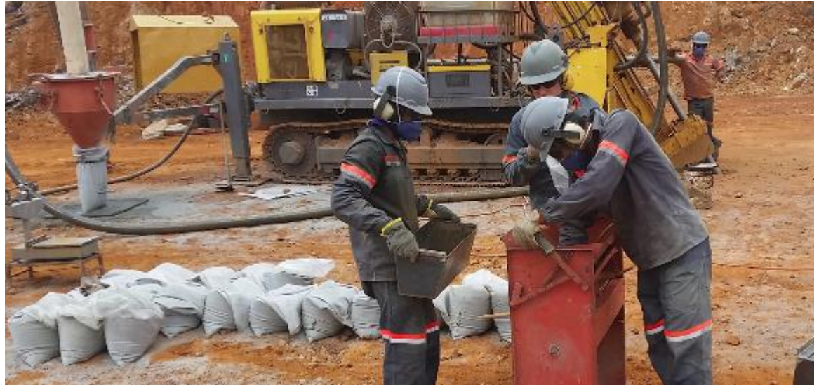
Cleaning splitter for sample preparation
