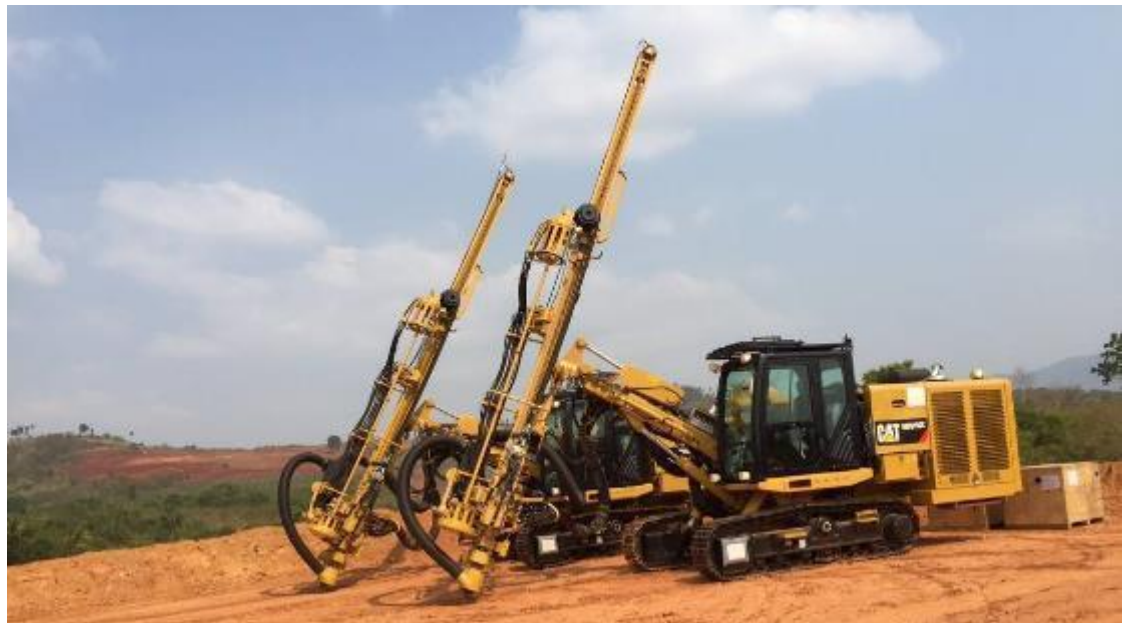
Delivery of Cat 5150C production drill rigs
