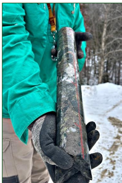
Figures 1-3: CDH001– visible chalcopyrite in chloritized felsic tuff unit @ 84.25 – 84.7m (refer to table 2)
