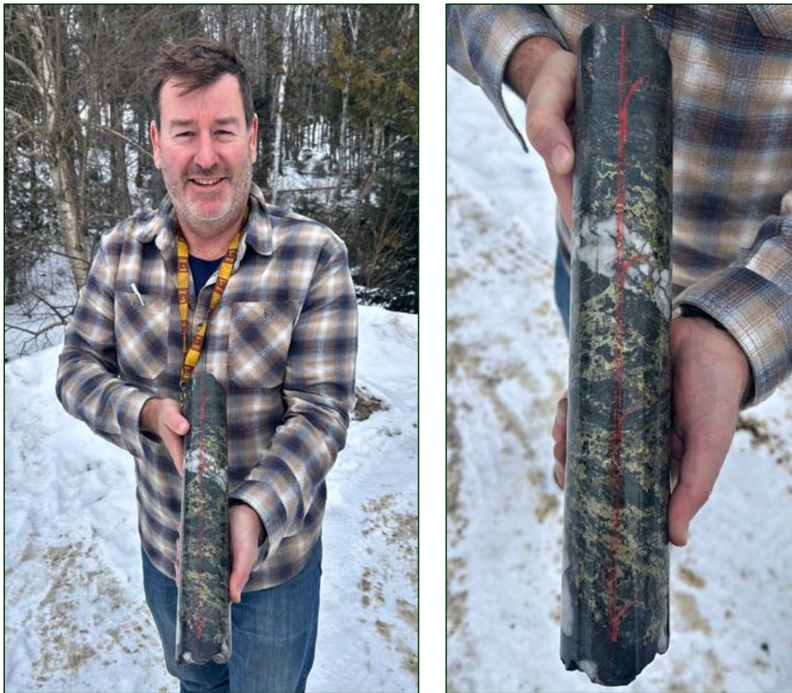
Figure 4 & 5: CDH002– visible chalcopyrite in chloritized felsic tuff unit @ 126.5m – 126.87m (refer to table 2)
