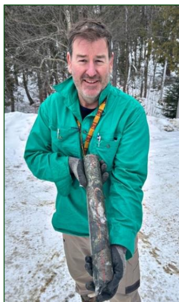
Figures 1-3: CDH001– visible chalcopyrite in chloritized felsic tuff unit @ 84.25 – 84.7m (refer to table 2)
