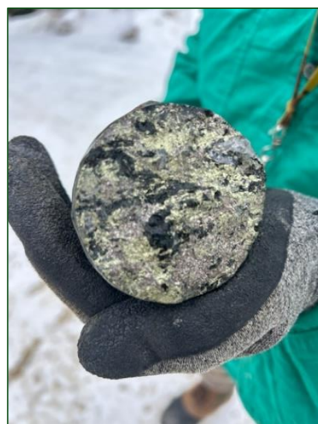
Figures 1-3: CDH001– visible chalcopyrite in chloritized felsic tuff unit @ 84.25 – 84.7m (refer to table 2)
