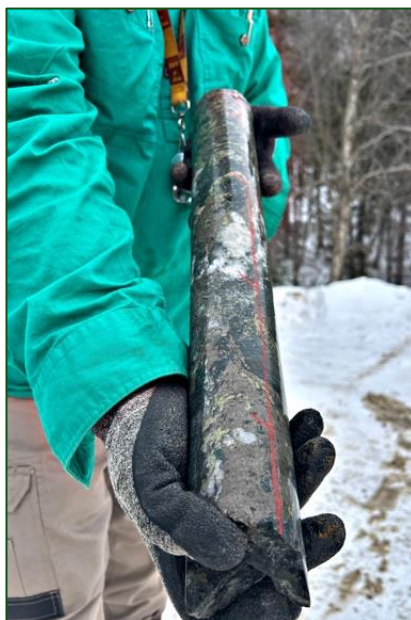
Figures 1-3: CDH001– visible chalcopyrite in chloritized felsic tuff unit @ 84.25 – 84.7m
