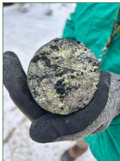
Figures 1-3: CDH001– visible chalcopyrite in chloritized felsic tuff unit @ 84.25 – 84.7m
