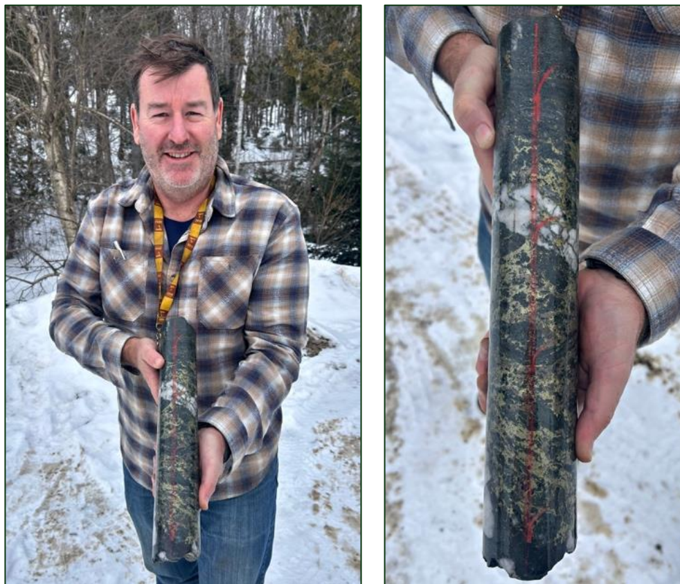
Figure 4 & 5: CDH002– visible chalcopyrite in chloritized felsic tuff unit @ 126.5m – 126.87m
