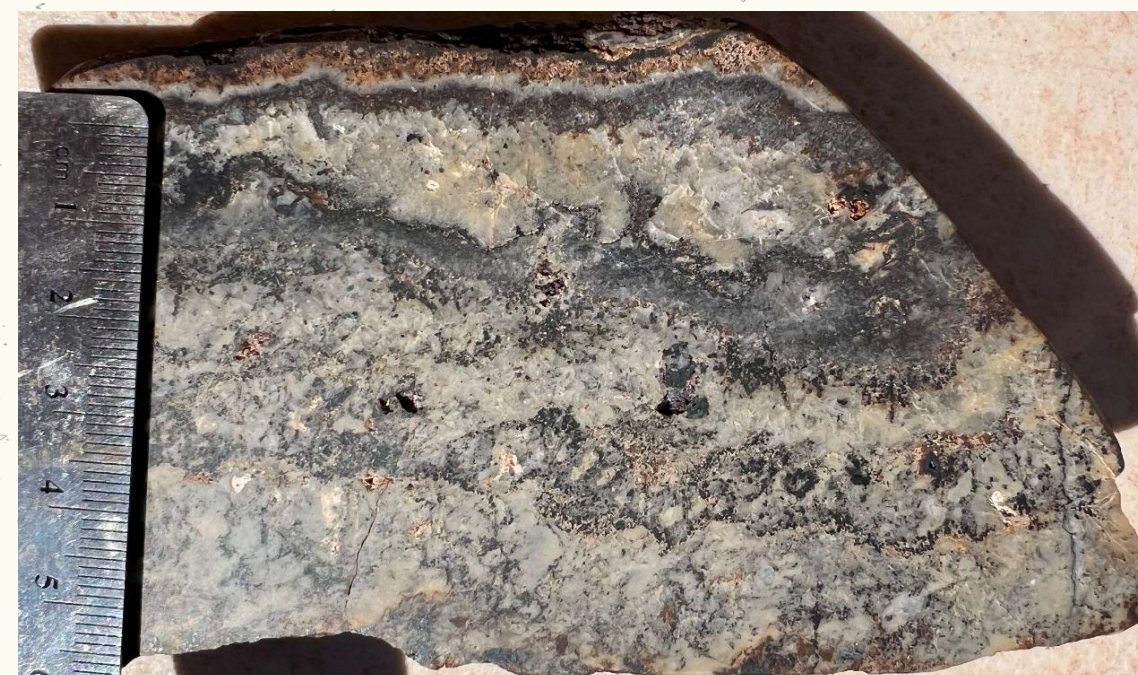
MHRK001 Colloform-crustiform quartz veining from the Mt Solitary prospect
