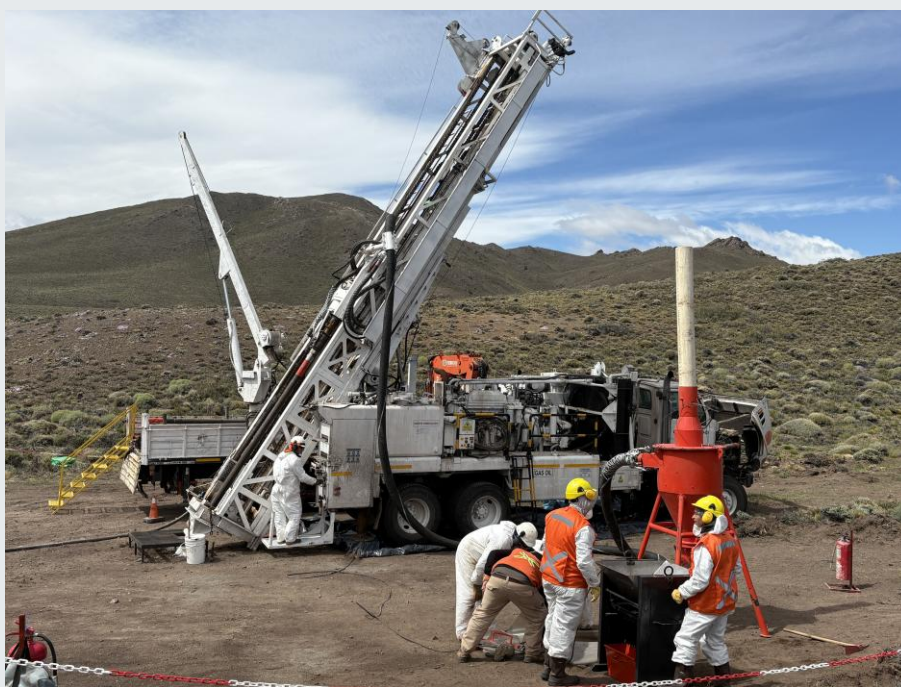
Figure 1: Reverse circulation drilling underway at the Cerro Chacón Gold–Silver Project, Chubut Province, Argentina (December 2025).
