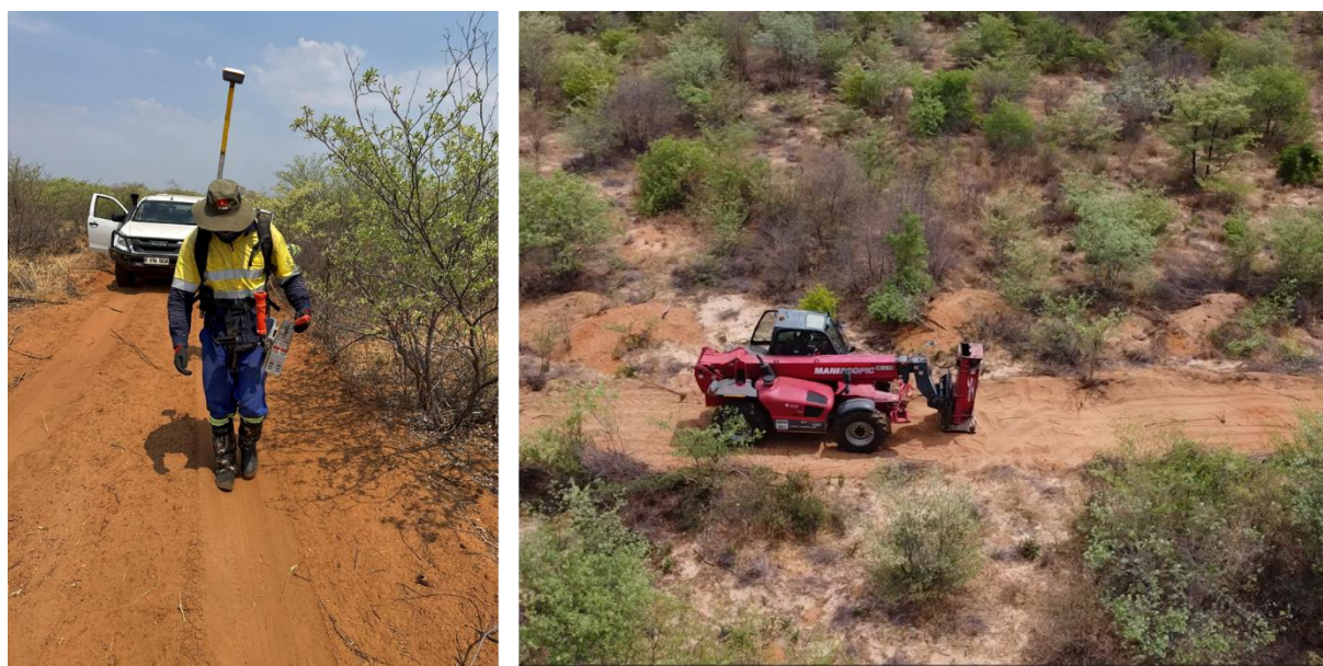
Figure 6. Seismic node deployment (left) and weight drop (right), Kitlanya West.
