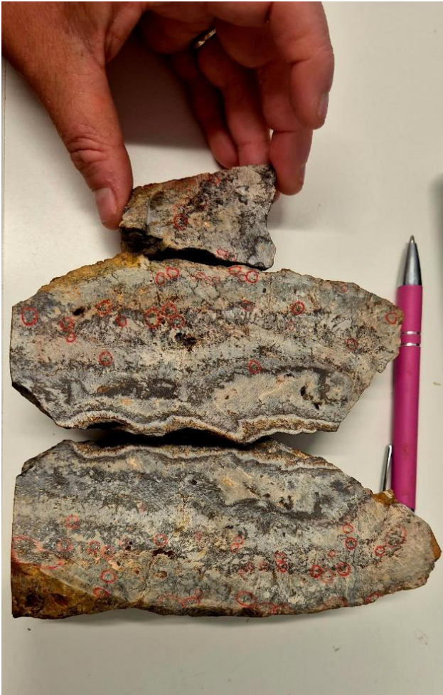
Figure 1: MHRK001 sample with colloform–crustiform banded texture and visible gold in red circles MHRK001: 40.89g/t Au, 4.45g/t Ag & 10,000ppm Bi
