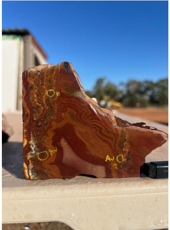
Figure 2: MHRK002 sample with colloform–crustiform banded texture and visible gold in yellow circles MHRK002: 52.5g/t Au, 1.15g/t Ag & 3,620ppm Bi
