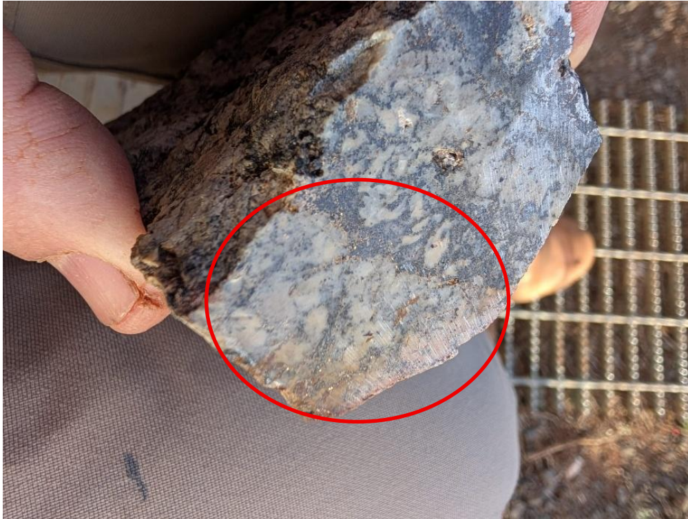
Figure 3: MHRK001: Close-up of Visible gold in iron & bismite banding, bottom half of sample
