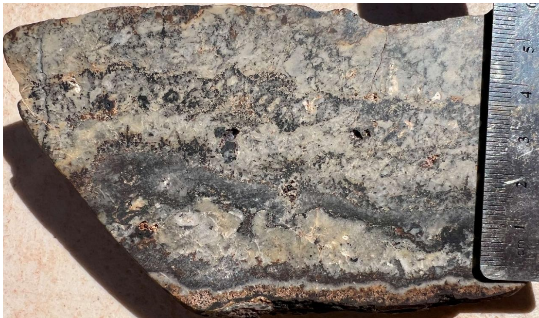
Figure 7: MHRK001 Coliform-crustiform quartz veining from the Mt Solitary prospect
