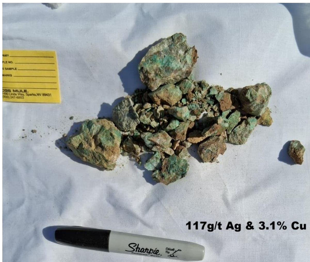
Figure 3: Rock Chip Sample 258420 – Malachite-stained selvages along a 50cm wide quartz vein
