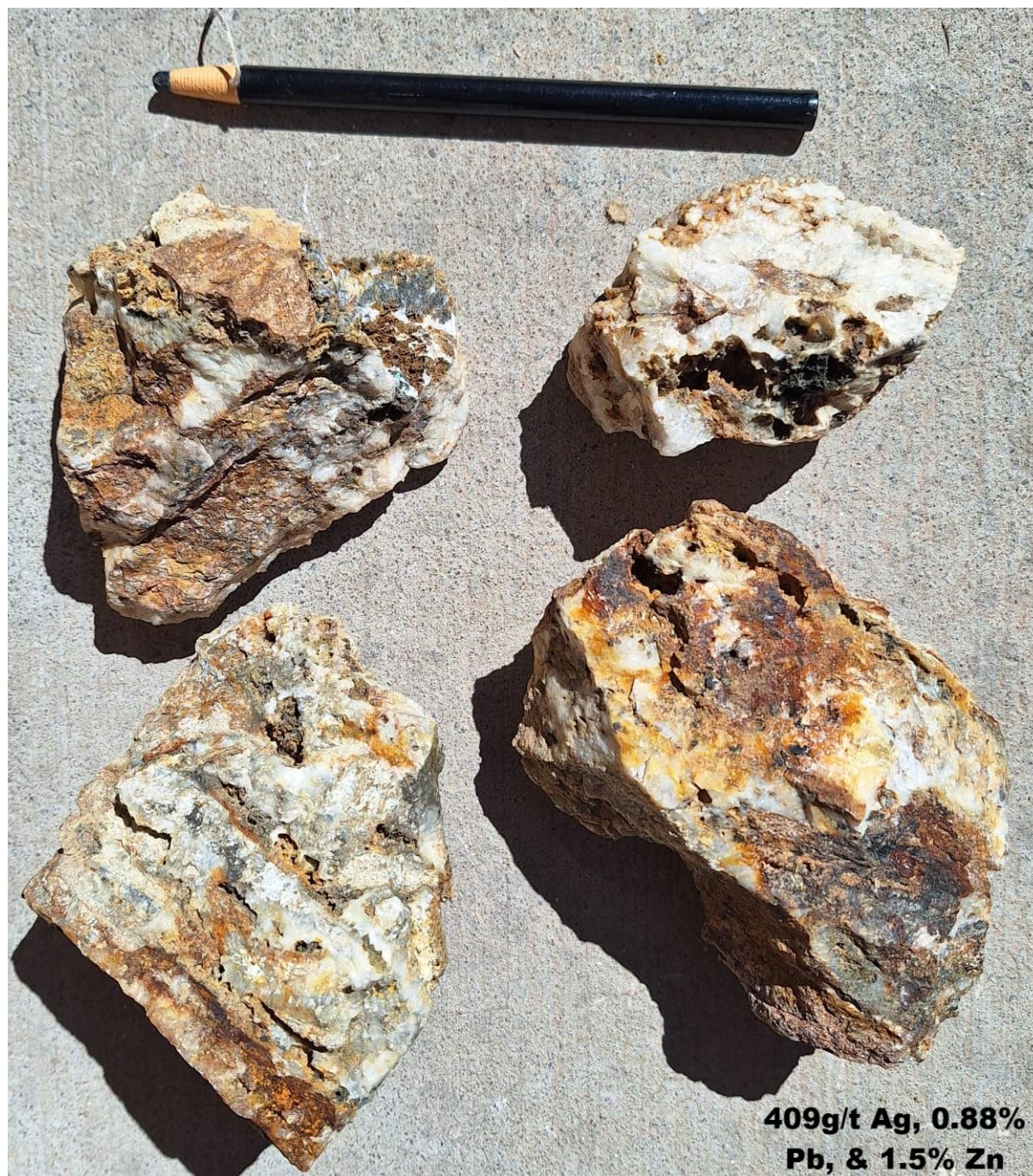
Figure 2: Rock chip sample 258185 which returned 409 g/t Ag, displaying gossanous textures indicative of weathered sulphides collected from historic stockpile containing gossanous selvages and boxwork textures
