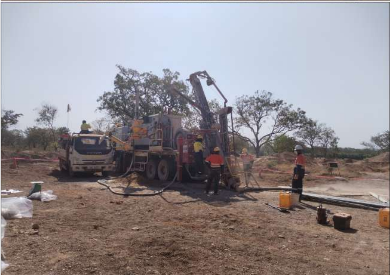
Figure 5: Sahara AC drill rig operating during Phase 2 strike extension drilling at Massan.
