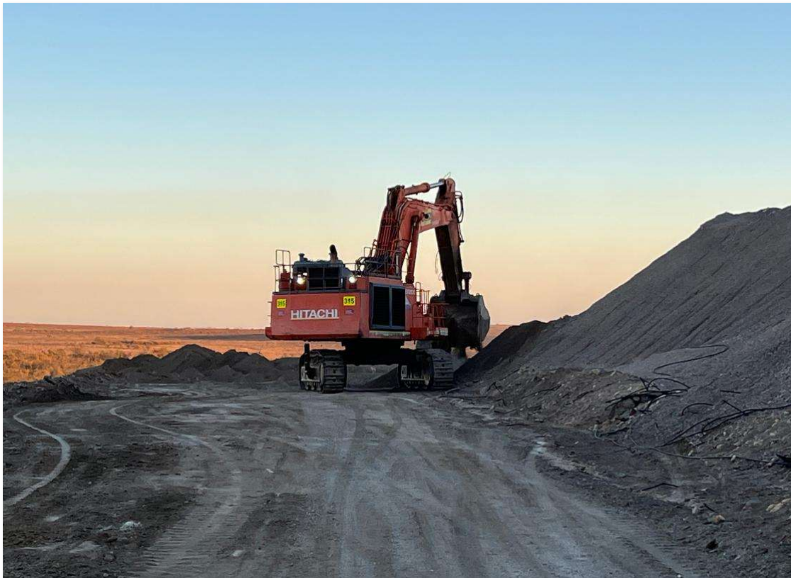
Figure 1; The recently mobilised 120T excavator working on northern berm of Heap Leach pad
