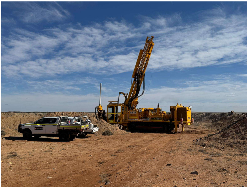
Figure 4; Vertigo RC Drilling underway at the White Dam Gold Project, South Australia
