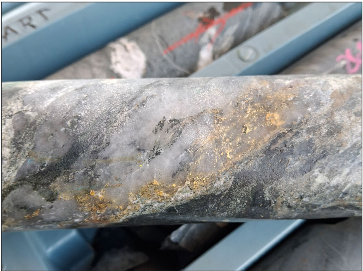
Figure 1: Visible gold in a quartz vein at 259.3m from hole 25HBBD024. The interval grades 0.3m @ 5848g/t Au from 259.17m (refer Table 1). 5 Core width is NQ2 and ≈ 50.5mm in diameter for scale.
