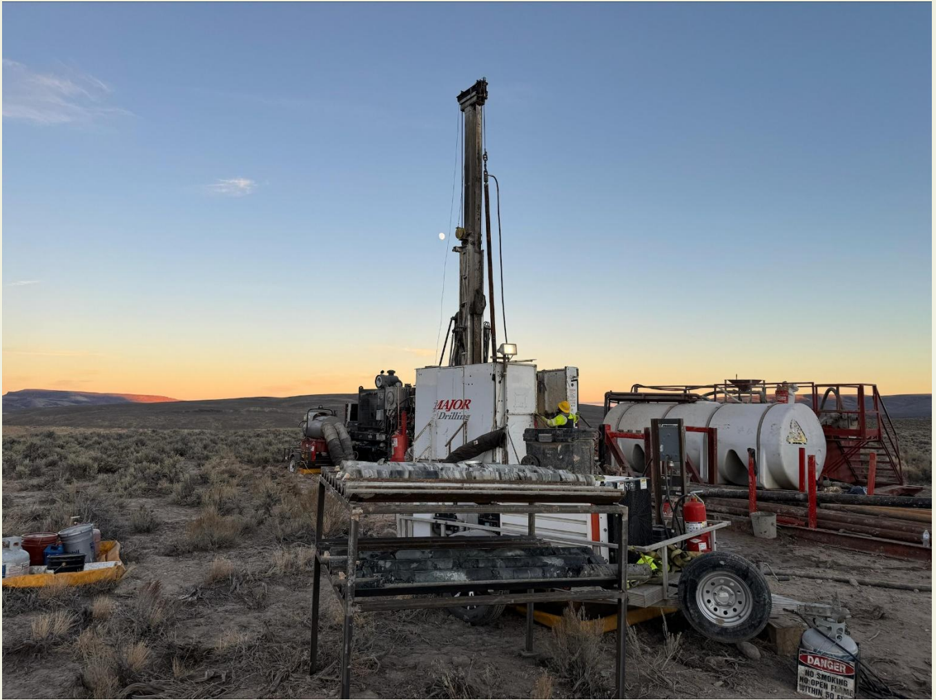
Figure 1 – Core Drilling underway at McDermitt
