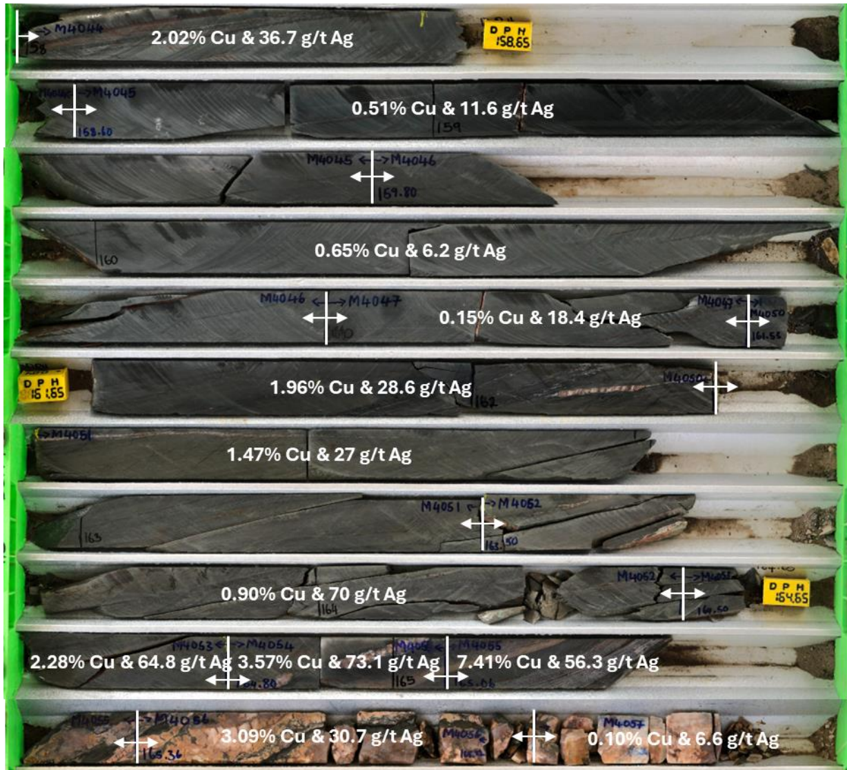
Figure 4. Drill core photos (HQ3 core) from NCP55 with sample results overlain. Note the increase in mineralisation towards the redox contact at the base of the figure with significant copper – silver assay values. See ASX Announcement 3 February 2025 for full JORC Tables related to the drill results from this hole.
