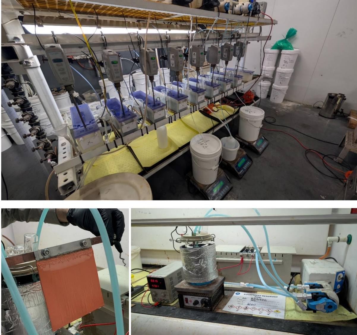
Figure 3. Solvent extraction configuration (top), derived copper cathode (bottom left) and electrowinning circuit (bottom right) from the bench tests.
