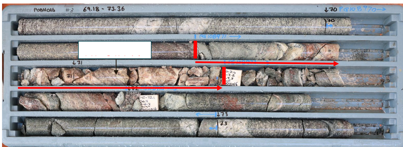
Figure 6: Posie Prospect drillhole PODH016 displaying quartz veining containing high grade gold: 0.86m @ 42.3g/t Au from 70.54m downhole depth
