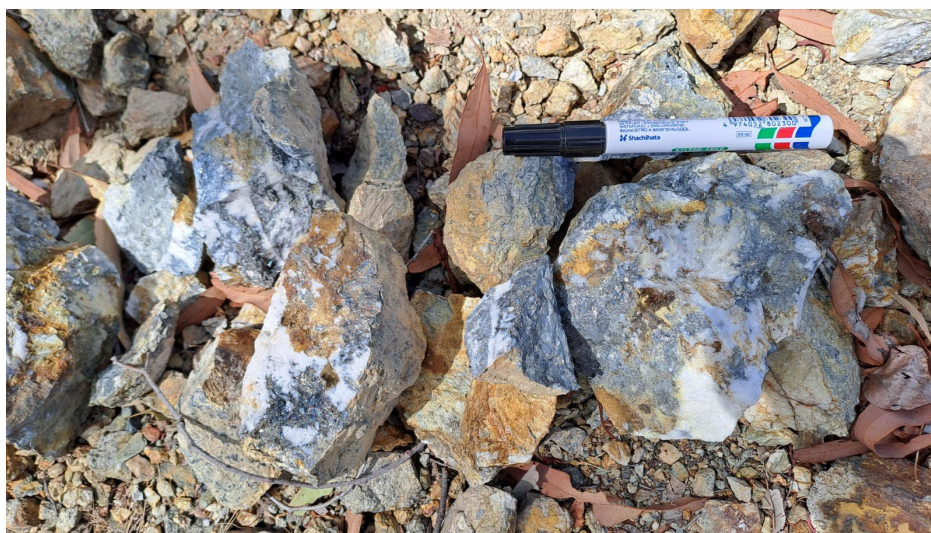
Figure 24: Rock chip samples collected from outcrop at the Poppy Prospect showing quartz with massive Stibnite (Grey Sulphide)
