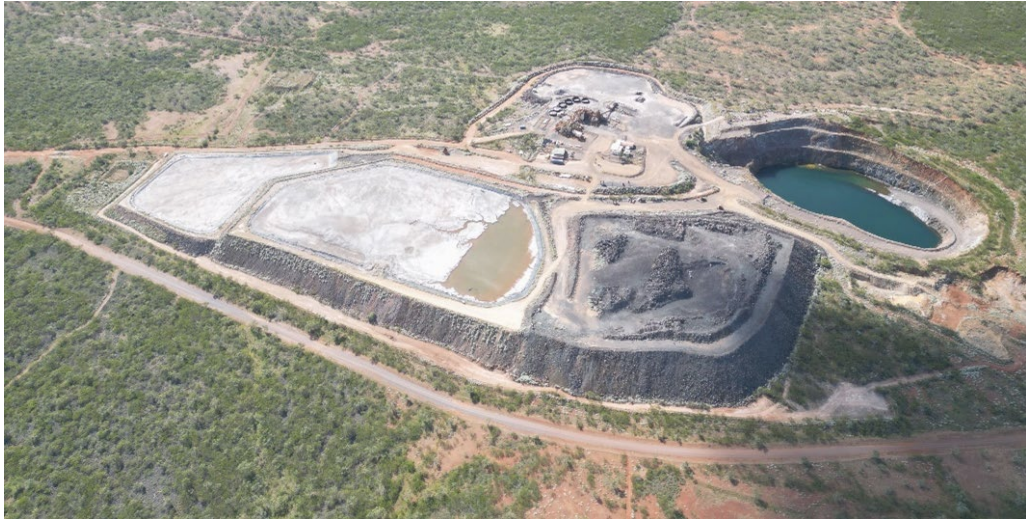
Figure 2 – Overhead of Lorena plant, tailings and waste rock stockpiles and open pit
