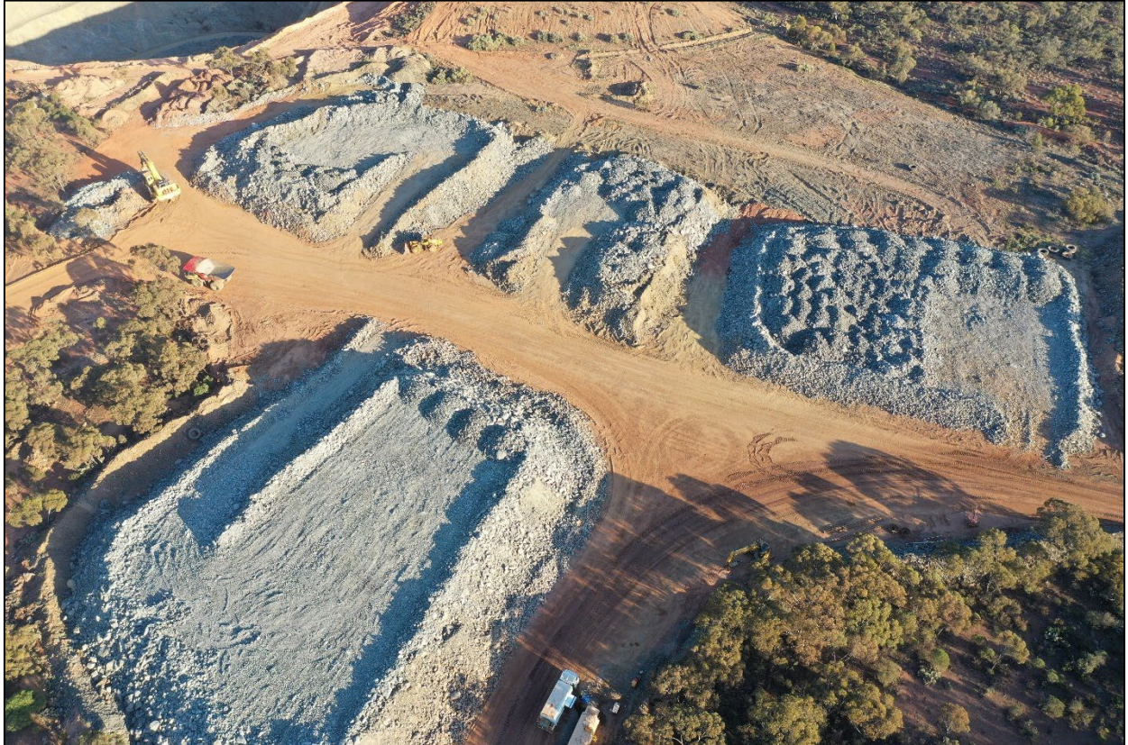
Figure 3: Ore on the Phillips Find ROM pad.
