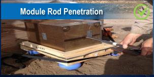
Fully charged Altech SNC battery pierced with 20 mm rod; water added. External reaction after 23 min produced steam, and minor HCl smoke over 4 h.
