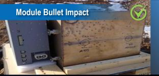
Fully operational Altech SNC battery hit by shotgun and rifle rounds; only minor smoke, no fire or explosion.
