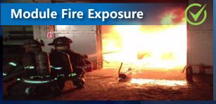
Hot, fully charged Altech SNC battery endured 30 min gasoline fire (850°C). Extinguished in 1 min with 3" hose. No explosion; case remained intact, minor mechanical weakening only.
