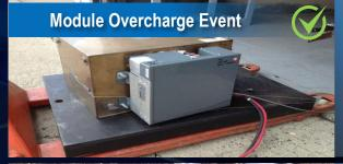
Fully charged Altech SNC battery exposed to 145% nominal voltage for 1 h (45% beyond UL1973)—no adverse effects.
