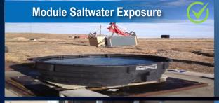
Fully operational Altech SNC battery exposed to 3.5% saltwater, including 2.5 h immersion. No fire or explosion.
