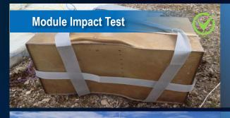
Fully charged Altech SNC battery packs impacted a simulated utility pole at 48 km/h in a vehicle. No explosion or fire occurred.
