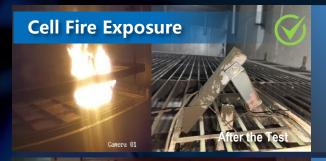
Three fully charged hot Altech SNC battery cell exposed to 30 minute gasoline fire. Fire temperature reached 850°C. No explosion. Cell case did not rupture. No emission of cell internal contents.
