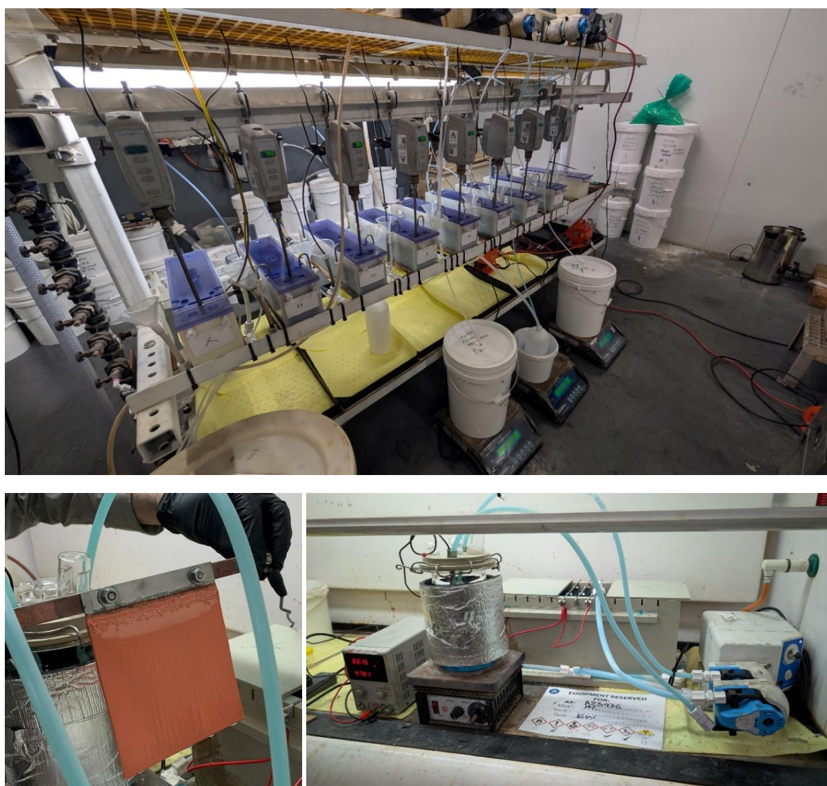
Figure 1. Solvent extraction configuration (top), derived copper cathode (bottom left) and electrowinning circuit (bottom right) from the bench tests.
