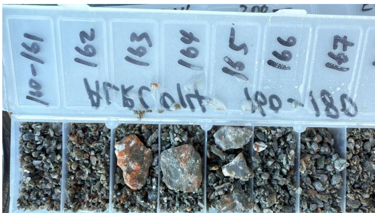
Figure 2: ALRC014 interval 160m - 167m averaging 1.58g/t Au
