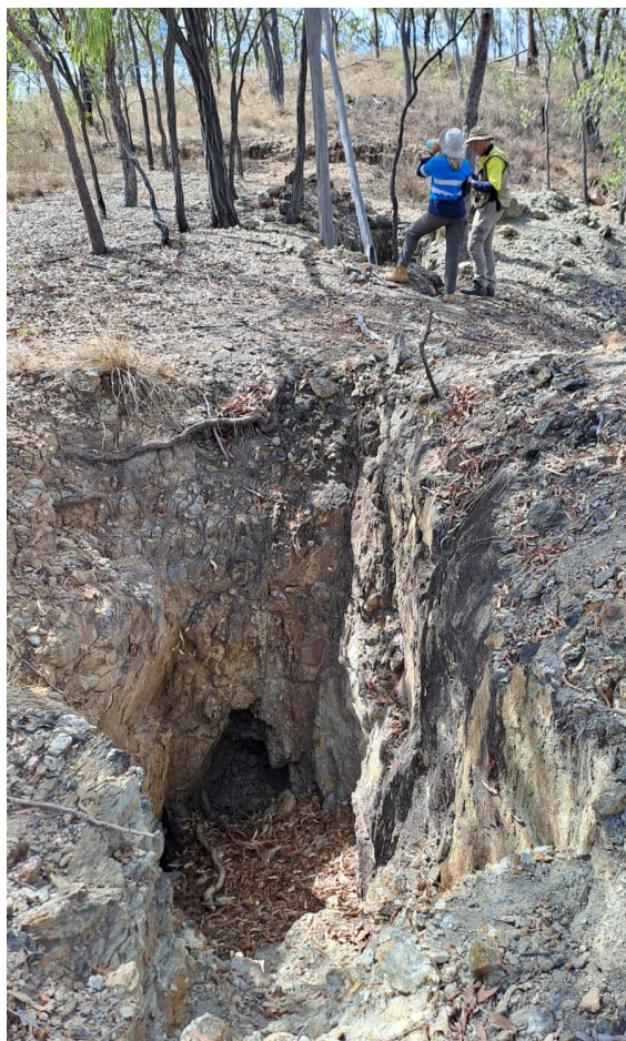
Figure 1: Pacgold Exploration Geologists at the Poppy Prospect artisanal Au-Sb mine, with adit and brecciated mineralised outcrop visible above entry to historic mine. The excavation extends down to approximately 30m below surface.
