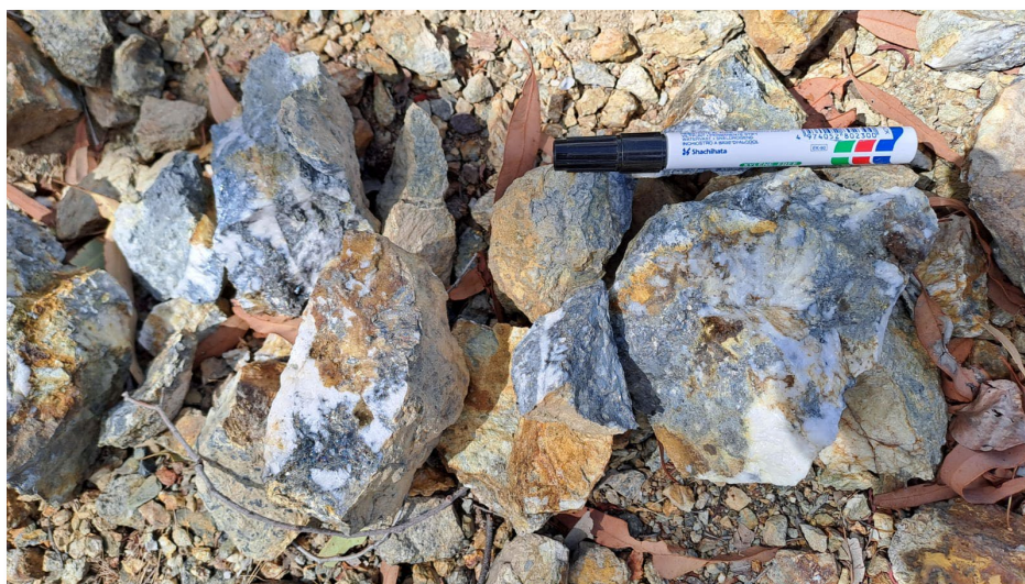
Figure 2: Rock chip samples collected from outcrop at the Poppy Prospect showing quartz with massive Stibnite 1 (Grey Sulphide)
