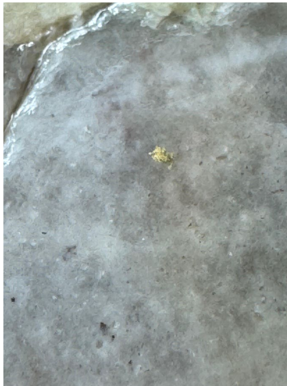
Figure 2: Visible gold from Posie drillhole PODH016, multiple occurrences of 1-2mm in diameter sized flecks were identified in core mineralisation very similar in style to the brecciated F1a zone at the Central Target. Refer to Figure 1 for core location.
