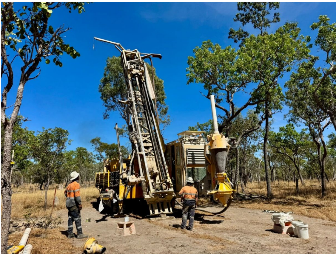
Figure 1: WLRC0001 hole location with RC drill rig being set up over site
