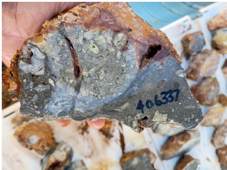
Plate 1: Sample 406337 Two stage breccia showing clasts of banded brecciated epithermal quartz assaying 3.72 g/t Au & 55.38 g/t Ag and Costean sampling at Tabu's Camp Prospect.
