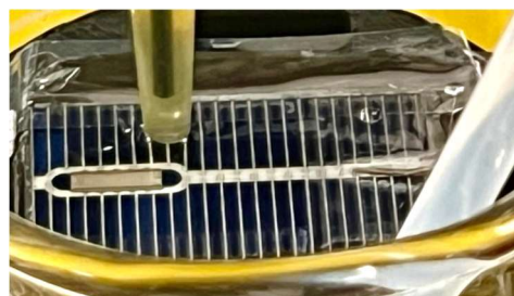
Figure 6 – Operation of the Electrochemical Jet Nozzle with silver dissolution
