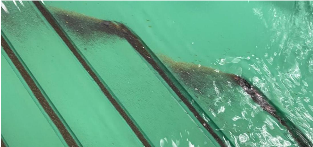
Figure 4 Coarse free gold recovered by gravity on the Gemini table at the Reward Gold Mine. The gold is being won from pre high grade underground production processing of the low-grade stockpiles.
