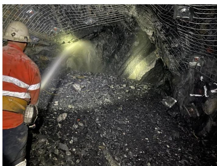
Figure 1 –Lady Belmore Reef being charged up and hosing down the ore (post blasting).
