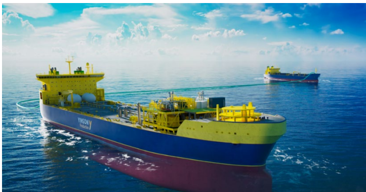
Illustration of a FSU in the foreground, receiving cargo from a LCO2 carrier in the background (Source: Yinson Production AS)
