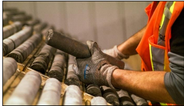
Image 3: Core tabled for quick logging at Fermont processing facility & 4: Core inspection in progress
