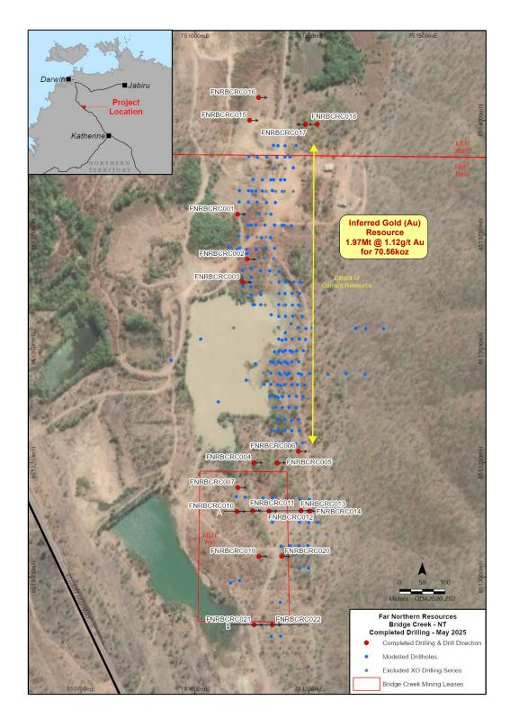
FIGURE 1: PLAN OF COMPLETED DRILLING – BRIDGE CREEK – PHASE 1
