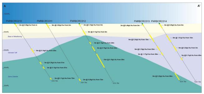
FIGURE 4: CROSS SECTION (A-A') LOOKING NORTH ~20M SECTION VIEW, SHOWING INTERPRETED GEOLOGY AND SIGNIFICANT INTERSECTIONS (AU >0.10g/t). DRILLING RESULTS ARE DOWNHOLE WIDTH AND NOT TRUE WIDTH
