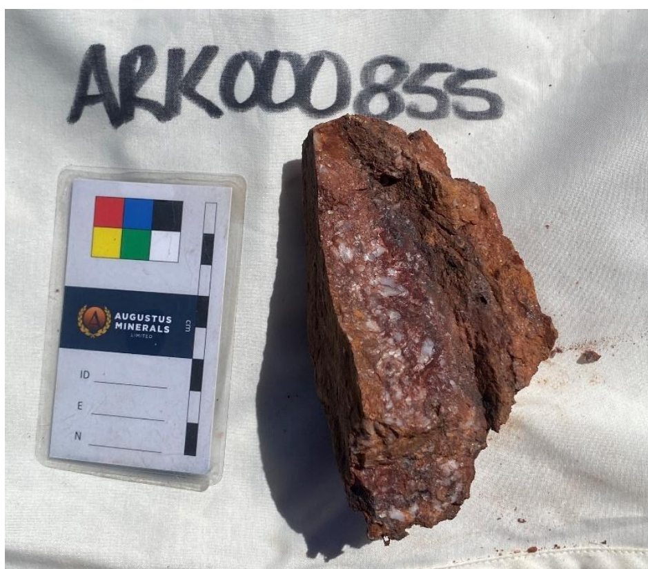
Figure 4 Rock chip of brecciated and gossanous quartz vein from the western extension of Clifton East prospect which assayed 7.99g/t Au.
