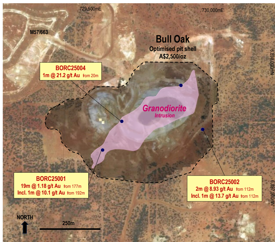
Figure 4 – Plan view map of Bull Oak drill collar locations (image within M57/663)
