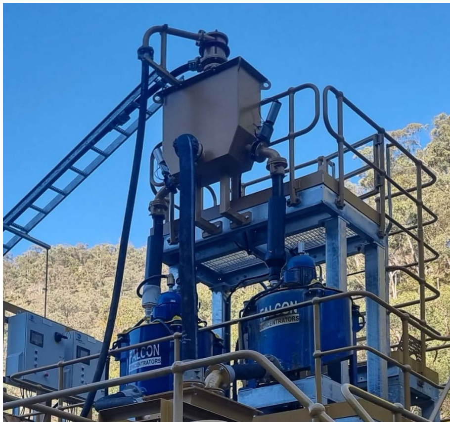
Figure 10 Reward gravity gold Falcon concentrators
