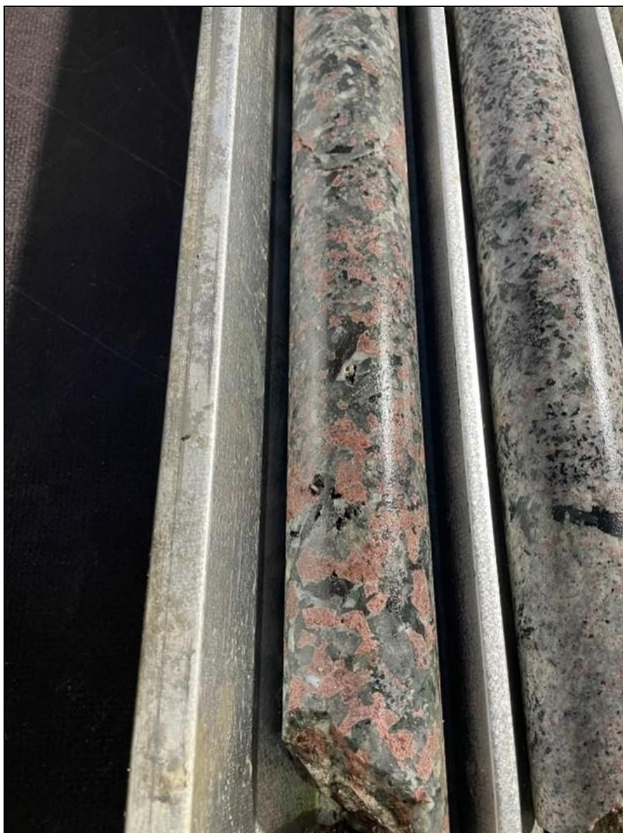
Picture 1 Drill core with high grade eudialyte from diamond drill hole A1-24 drilled September 2024 containing 4,722.51ppm (0.47% TREO) (including 26.96% HREO" and 101.67ppm Ga_2O_3 "gallium oxide".
