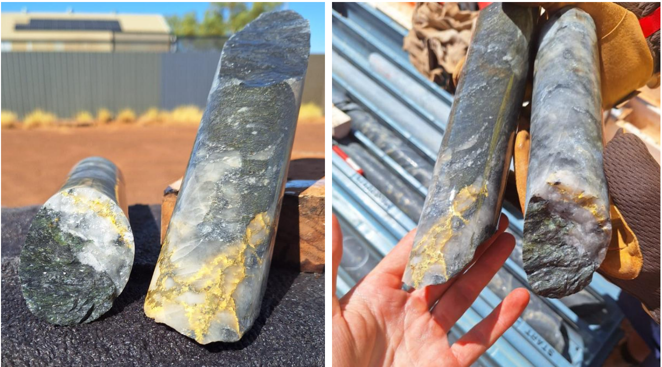
Photos 1 & 2: Visible Gold in Quartz - Carbonate Vein intersected at 252m down hole in NGGRCDD974 within a broader 16m wide shear zone.
