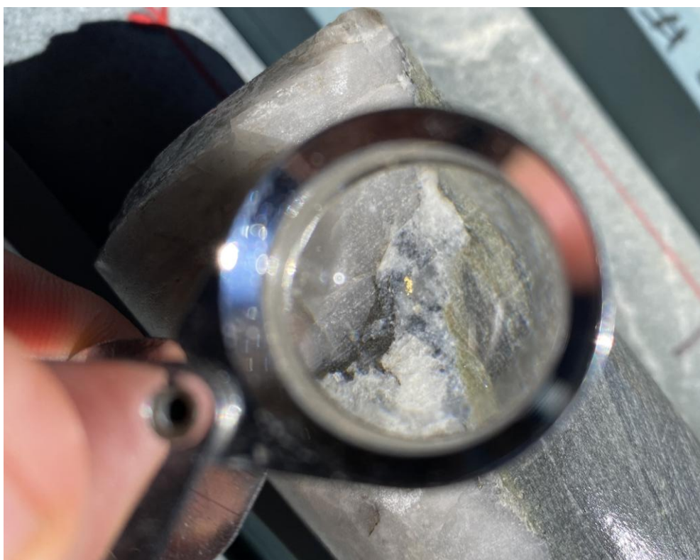
Photo 3: Visual free gold at 568m within Q-Carb vein in NGGRCDD980.
