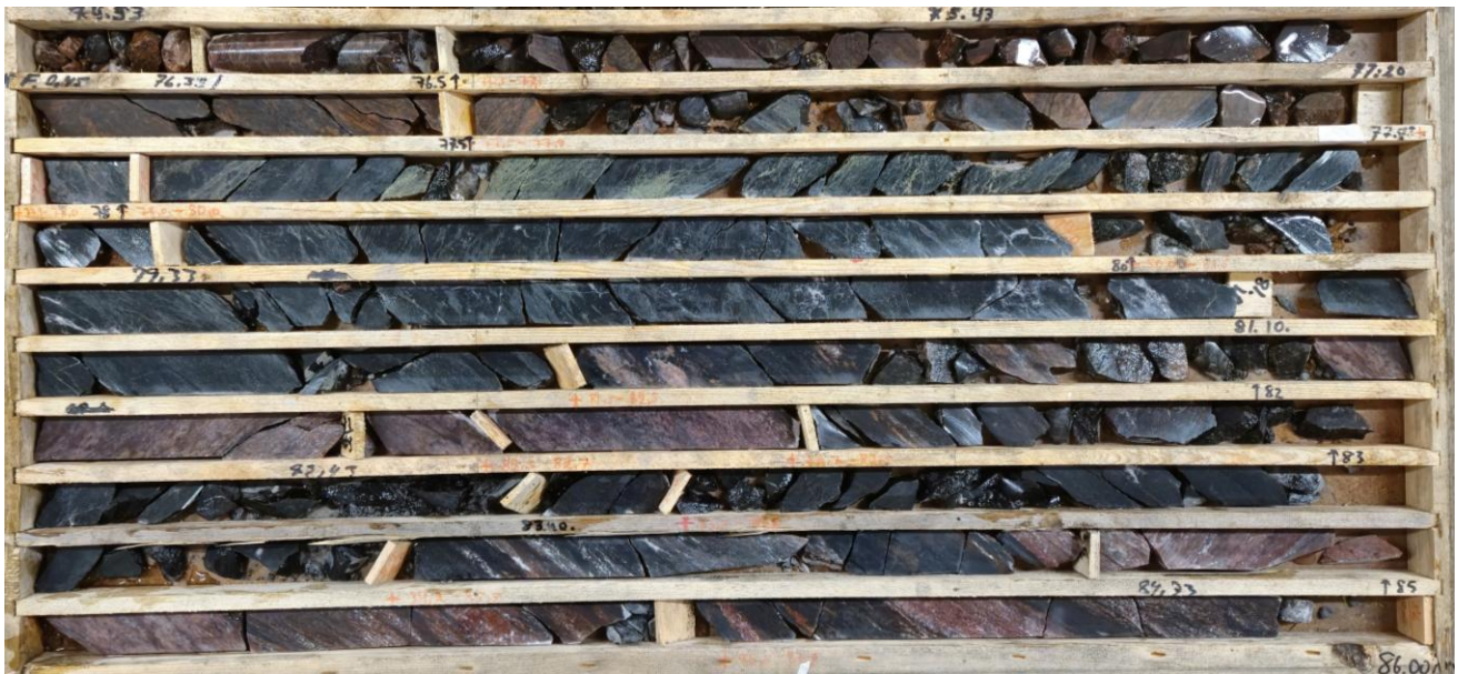
Figure 3: Core photograph of drillhole VIRKA80004 (76.2-86 m) (Virka) displaying mylonitic deformation and vein/fracture stockwork.
