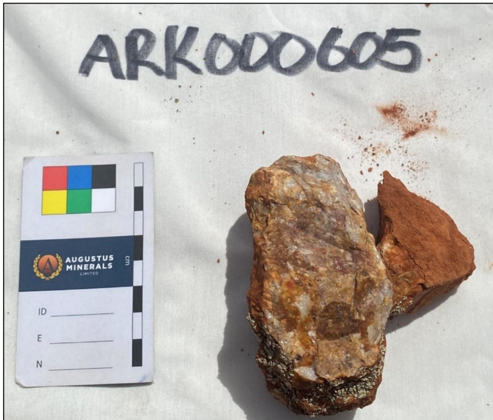
Figure 6 Rock chip assaying 21.3g/t Au quartz vein with iron oxides after sulphide from Clifton East prospect (sample ARK000605).
