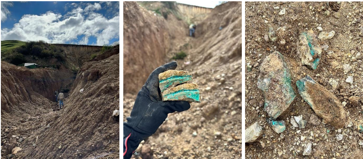
Figure 9: Left – Historic pit at Irka SW Porphyry-Skarn mined to 10m depth being investigated. Middle – Presence of supergene copper mineralisation of Azurite and Malachite at base of pit. Right – Further presence of highly enriched copper bearing ore present at base of pit.
