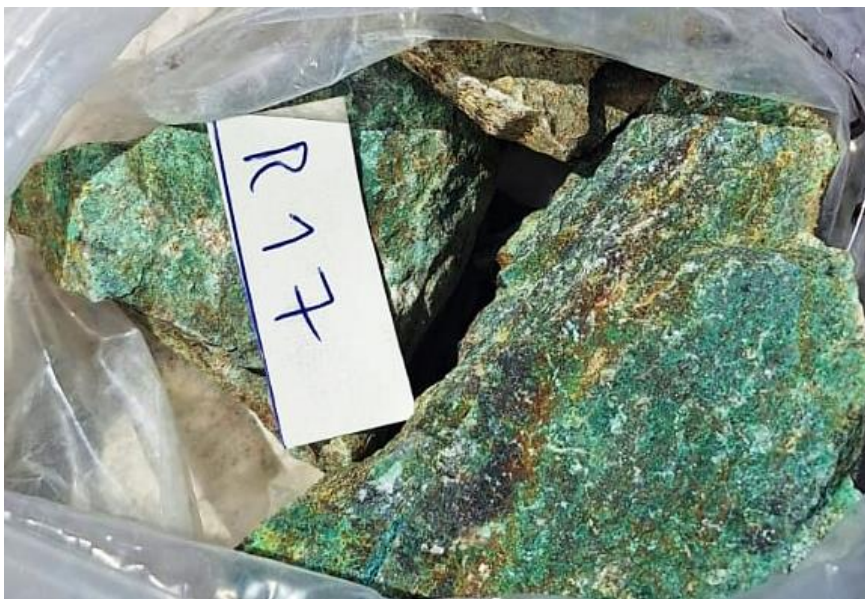
Figure 4: Sample R17 bagged, which returned 2.9% Cu, 0.24g/t Au, 92g/t Ag and is the furthest northwest sample taken at Irka Sur – 700m along strike (SE-NW) from Sample R28
