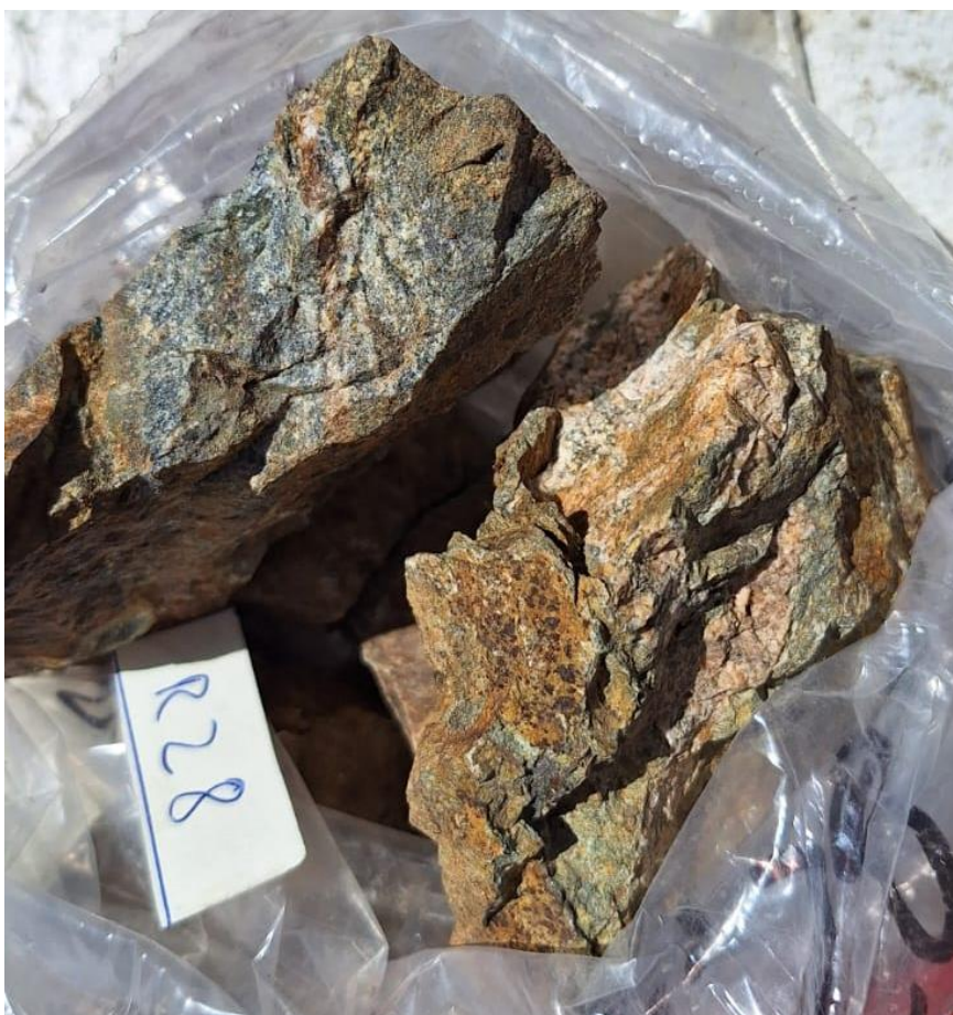
Figure 5: Sample R28 bagged, which returned 0.8% Cu, 0.29g/t Au, 63g/t Ag and is the furthest southeast sample taken at Irka Sur from outcrop. Sample was taken 700m along strike (SE-NW) from Sample R17 at a 140m lower elevation in the system.
