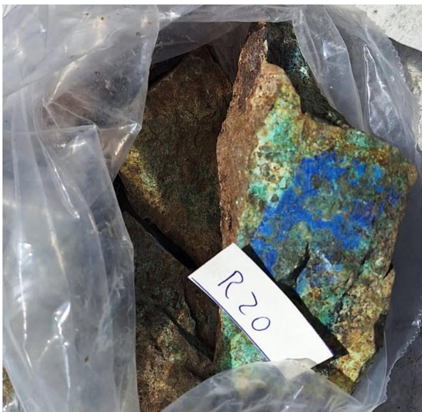
Figure 6: Sample R20 bagged, which returned 2.2% Cu, 0.14g/t Au, 105g/t Ag taken from outcrop present at Irka Sur with prominent Azurite present.
