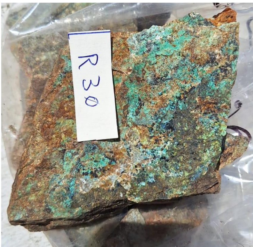
Figure 7: Sample R30 bagged, which returned 1.0% Cu and 14g/t Ag taken from outcrop present at Irka Sur.
