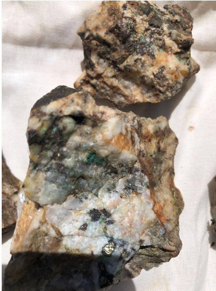
Figure 5: Sample P24654 with visible Malachite and Chalcopyrite
