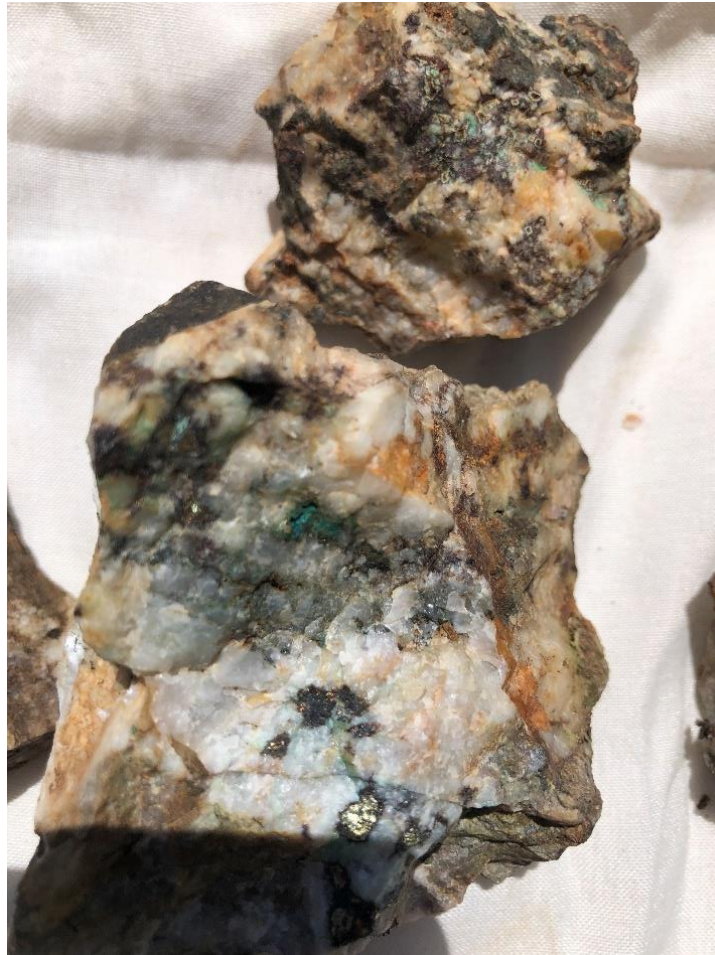
Figure 3: Sample P24654 with visible Malachite and Chalcopyrite
