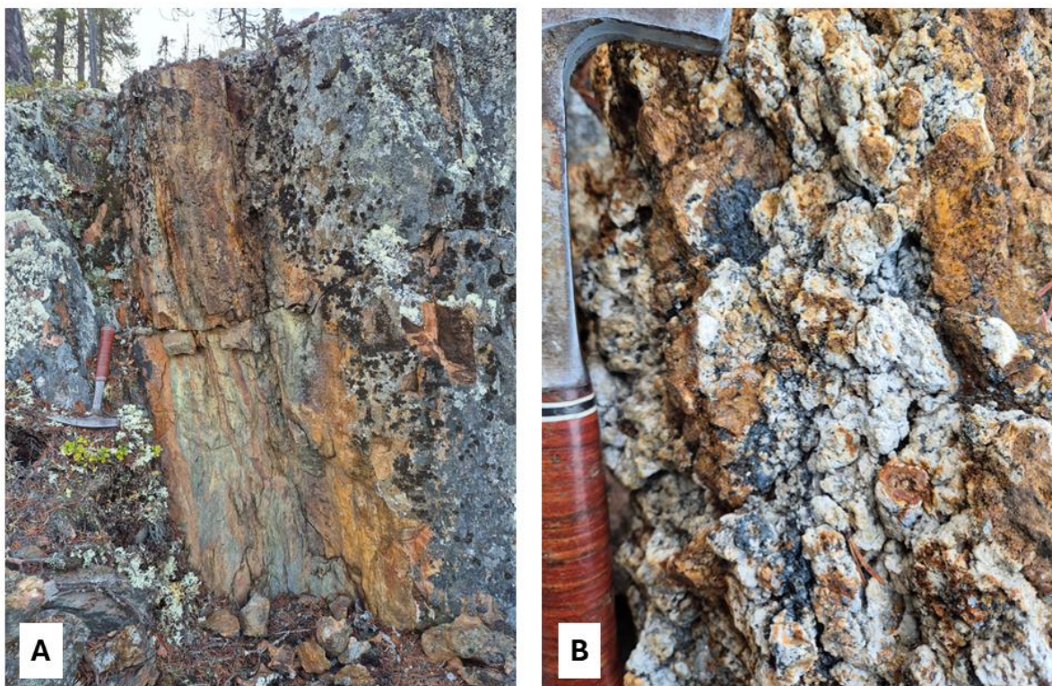
Figure 2A: Polymetallic vein outcrop at Virka. Refer VRK016, Appendix 2 for assay data
