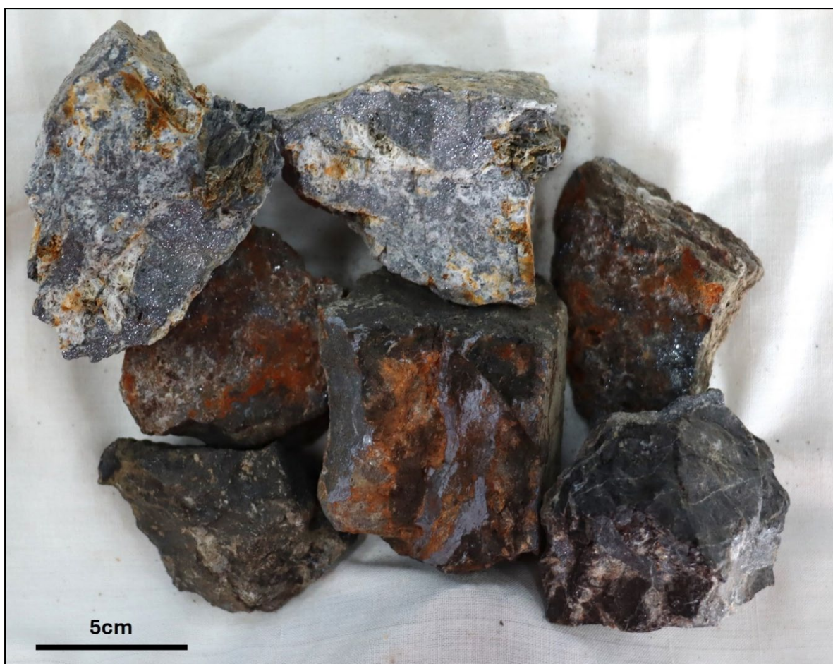
Figure 4 – High-grade silver-bearing galena mineralisation from rock sample AV018 which assayed 581g/t Ag with 36.5% Pb and 4.1% Zn.
