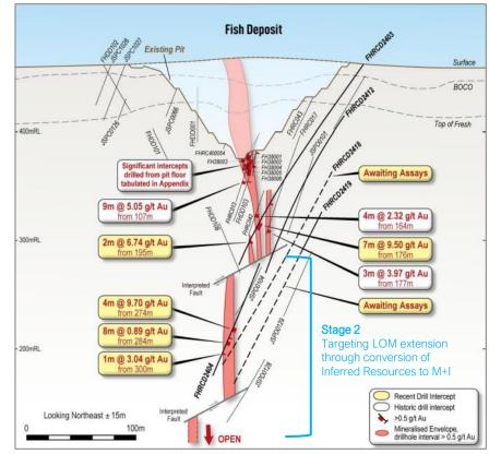
Fish cross section showing continuity at depth
