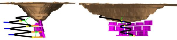
Scoping Study<sup>1</sup> designs beneath existing open pit Cross section looking north (left); long section looking east (right)
