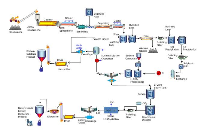
Figure 10: Lithium Universe Bécancour Process Flow Sheet
