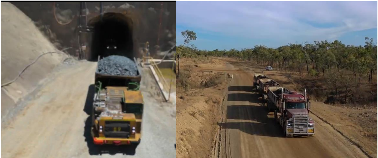
Figure 5. (a) King Vol Portal, (b) Road train used to haul King Vol 25 km from the King Vol mine to the Mungana Processing facility. Note that Tartana is the same distance as the King Vol mine to the Mungana processing facility. (source: Auctus Resources)
