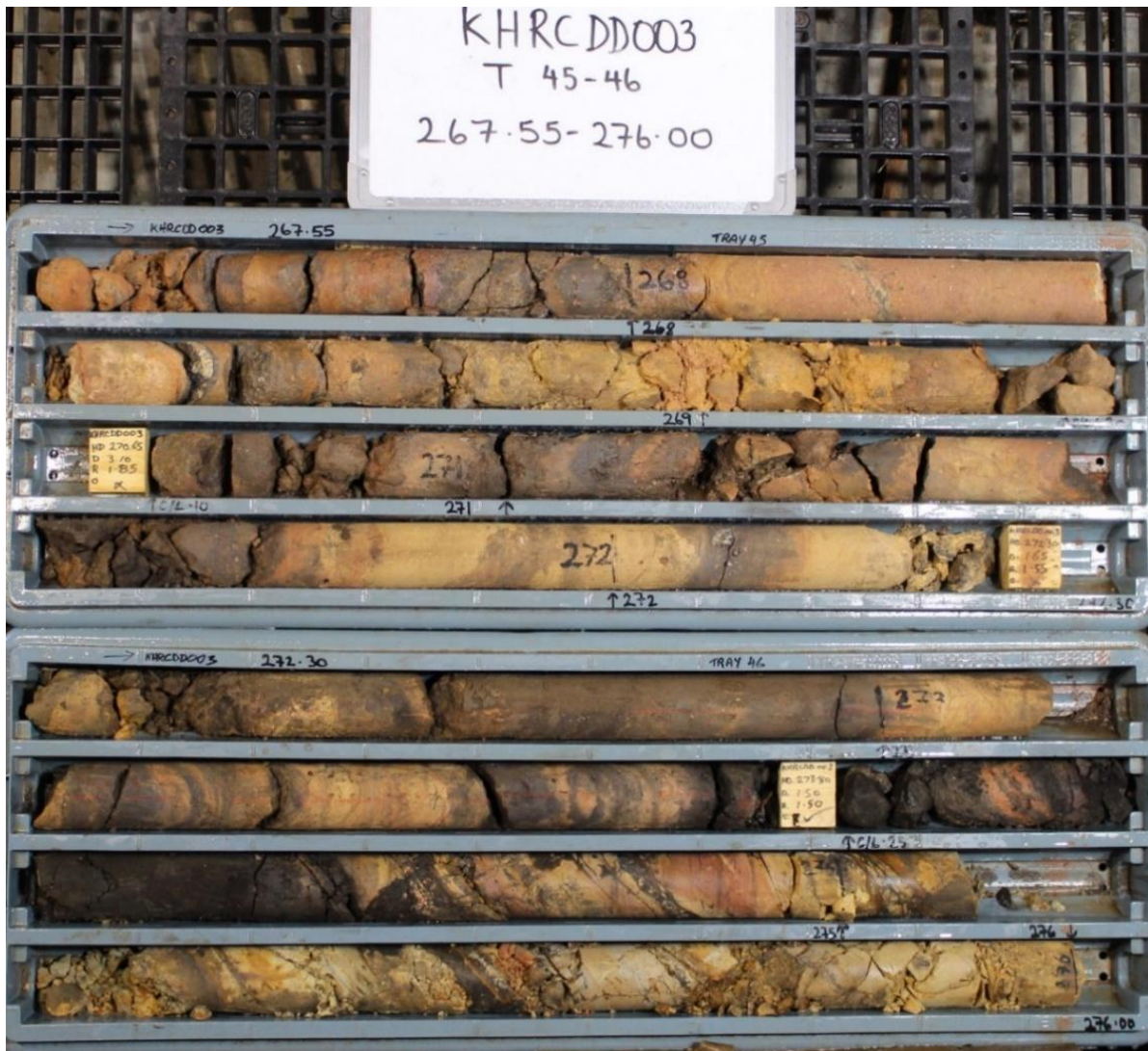
Figure 5: Ferruginous-gossanous oxidised Preston Formation sediments, KHRCDD003. Refer to Table 1 in ASX:EMS Announcement dated 23 October 2024 for assay grades.
