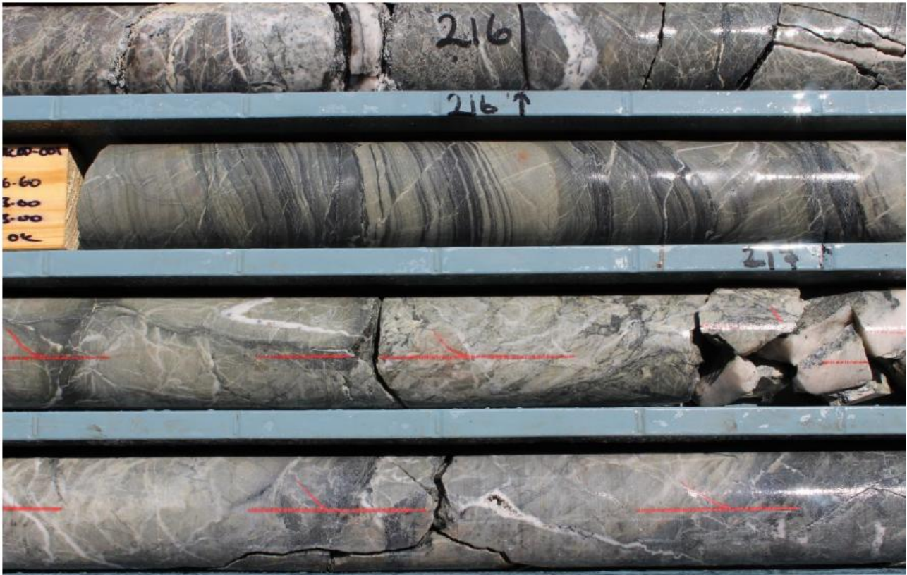
Figure 9: Intense texture destroying phyllic (silica-sericite) alteration present within WDRCDD001 from 215.62m to 218.93m.
