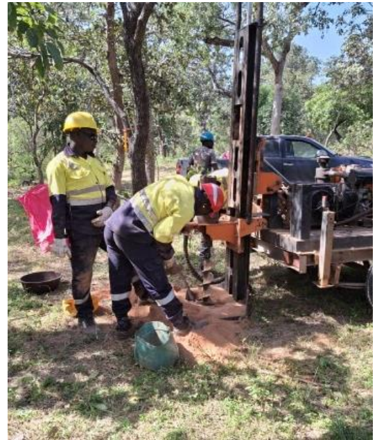
Figure 3 | Auger drilling at Ferké Gold Project
