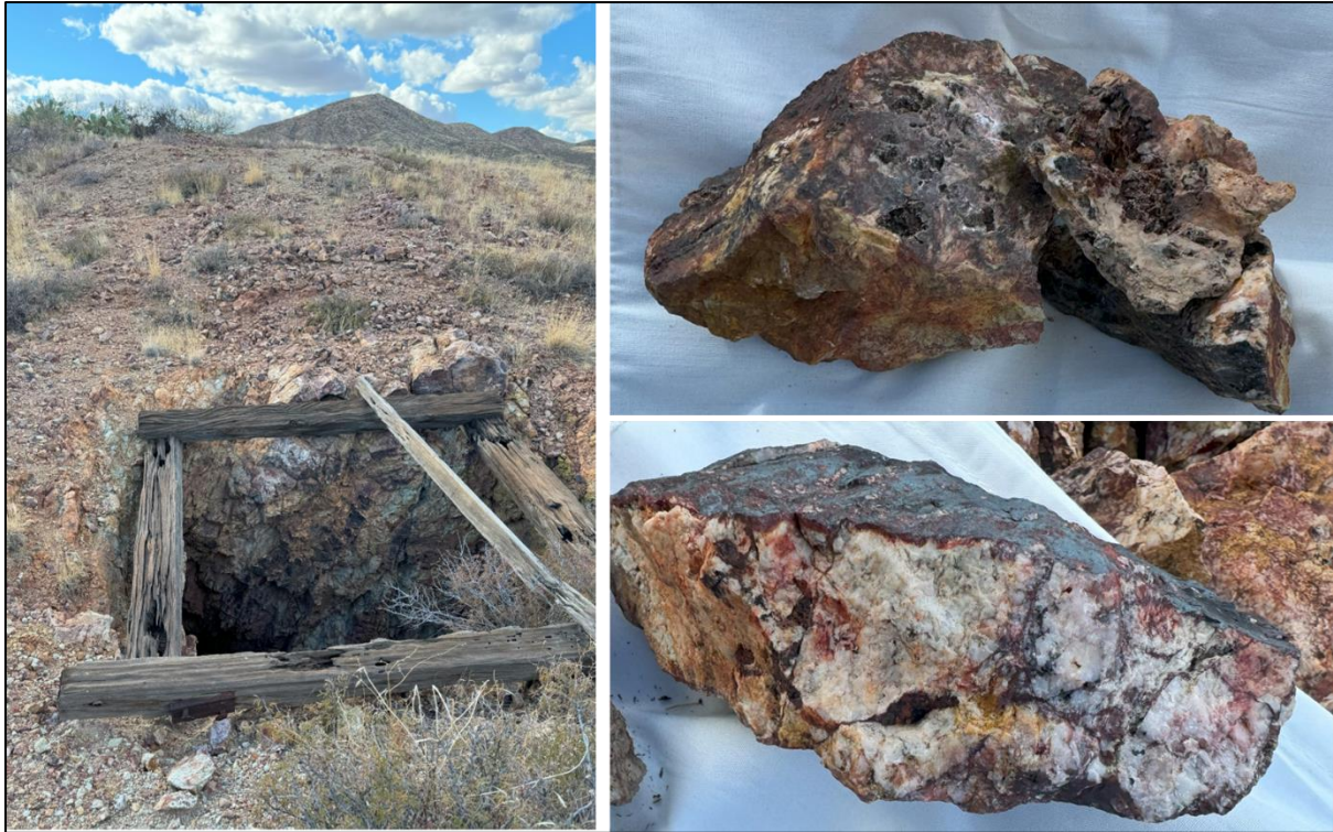
Figure 1: Aurora Prospect. Left: Gold mine shaft. Upper right 24PRL0126 10.8 g/t Au, 33.3 g/t Ag, 2.62% Pb. Lower right 24PRL0125 8.93 g/t Au, 22.3 g/t Ag, 0.11% Cu.
