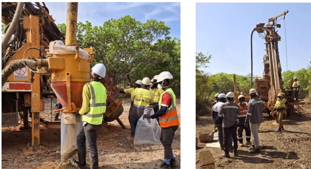
Figure 4 | Air Core drilling at the Odienné South Permit
