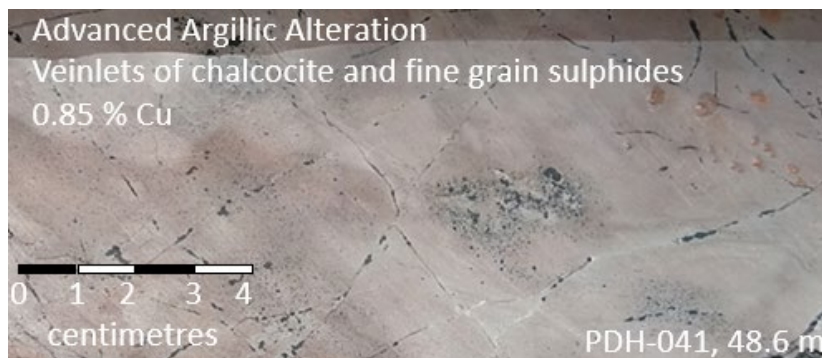
Figure 4-4: Advanced Argillic Alteration, Veinlets of Chalcocite and Fine Sulphides (Source: MA 2024)
