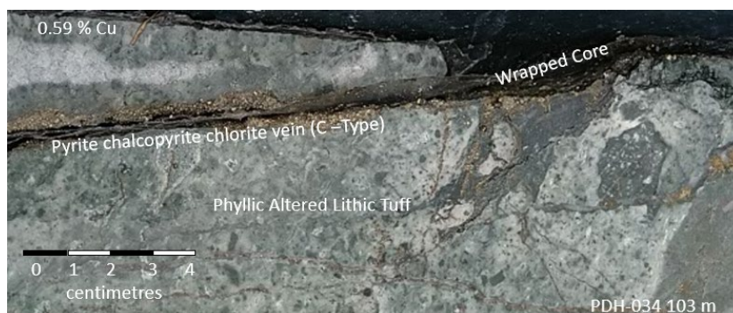
Figure 4-6: Phyllic Altered Lithic Tuff with A Pyrite Chalcopyrite Chlorite Vein (Source: MA 2024)
